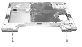
Figure 2-25 Remove the two screws
